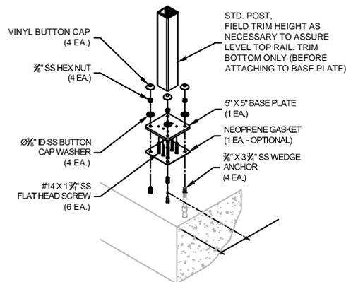
TYP. SURFACE MOUNT TO CONCRETE CONNECTION
